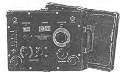
2-38 Twin-T Impedance Measuring Circuit GR Type 821 1940
